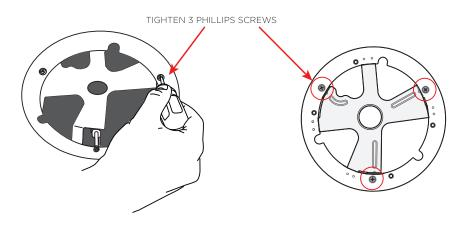
NOTE: If installing into drywall or ceiling tile; over-tightening the wings can damage the mounting surface, possibly leading to the camera falling, causing damage or injury.
