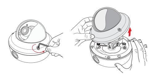
**b.** Remove the four Phillips head screws that hold the inner case onto the camera base, then remove the inner camera assembly from the camera base. Set this base aside. You will not need this base when using the Recess Mount.
