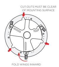
NOTE: When mounting make sure the mounting surface does not block the 3 perimeter cut-outs shown above. These cut-outs must be clear in order to accept the Vandal X case in the next steps.
