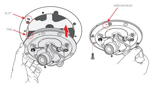
**b.** Replace the dome cover onto the camera assembly and tighten the 3 Torx screws to complete the installation. Make sure each screw is tight to ensure superior weather resistance.
