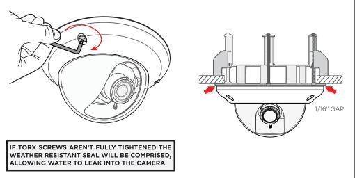
NOTE: Due to the replacement of the bottom case, a 1/16" gap between the Recess Mount and the Vandal X camera will result. This will not affect the IP68 weather rating of the Vandal X series camera.
