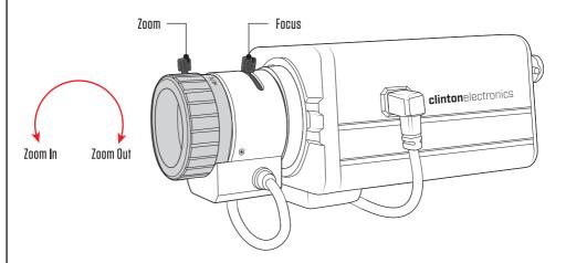
Actual lens ZOOM & FOCUS adjustments may vary from those shown. After adjustments have been made make sure to tighten the adjustment knobs to lock the adjustments into place.
