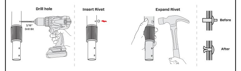
\*CE-CM-LX17 only: This pole requires two rivets to be inserted, one for each section of telescoping pole length. Repeat the steps above for each section of pole.
