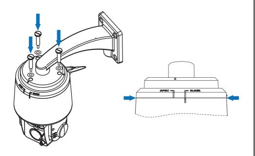
ATTENTION If locking bolts and washers are not used or aren't fully tightened the weather resistant housing will be compromised, potentially allowing water to leak into the camera.
