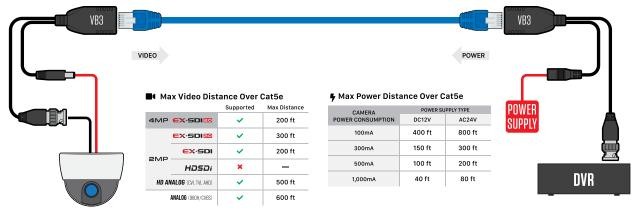
\*Distances shown based on new CAT5e ethernet cable. Distances will vary depending on camera signal type, power consumption, & ethernet cable type/integrity. Splices, couplers and severe kinks will reduce the overall possible distance.
