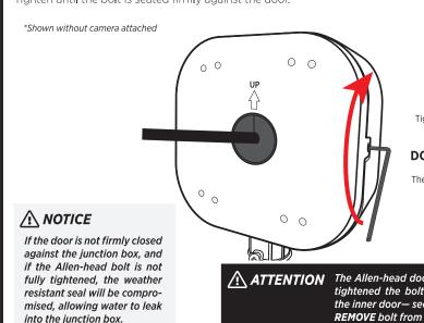
Tighten recessed Allen-head bolt until snug against inner door.
