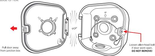
ATTENTION The Allen-head door bolt is reverse-thread. DO NOT REMOVE bolt from the junction box housing.
