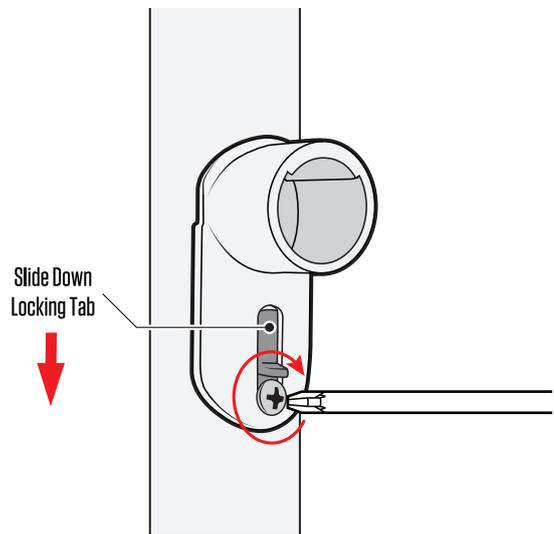
\*Ensure the raised tab is protruding from the slot, above the screw, in the bottom of the CE-TPCA Adapter.
