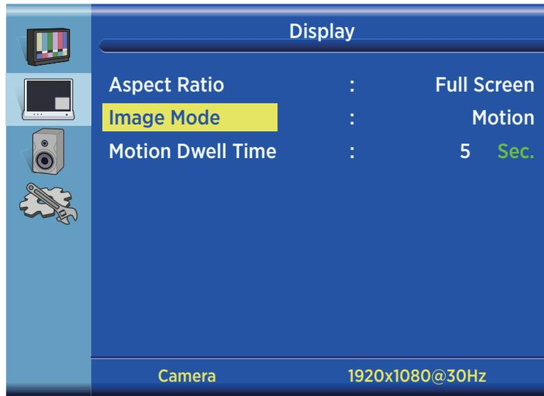
**Camera:** Only the camera image is shown on the screen of the PVM, no switching occurs.
