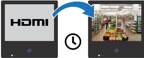
**Switch SD Video:** The screen will switch back-and-forth from the camera image to the SD Card content at set time intervals.
