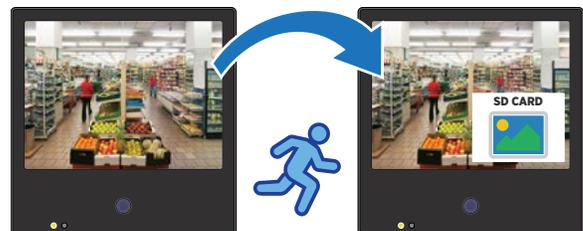
**Alarm VOV:** SD Card content will be full screen until triggered by the Alarm Input— when triggered, a “Return to Cashier” message will flash on the screen.
