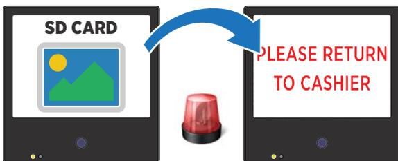
**Alarm:** The camera image will be on the screen until triggered by the Alarm Input— when triggered, a “Return to Cashier” message will flash on the screen.
