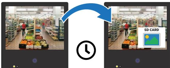
**Motion VOV:** The camera image will be full screen with no motion, when motion is detected by the PIR sensor the SD Card content will be shown over the camera in the corner of the screen.
