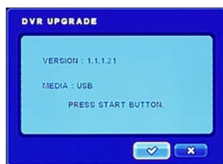
Confirm the firmware update by clicking the ✓ button, do not remove USB from DVR or power down
