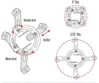
**OPTIONAL:** If desired, remove unused mounting arms depending on the number of mounting holes on the camera.
