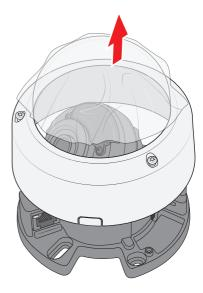
i NOTICE The 3 Torx screws are not designed to be fully removed from the dome top.
