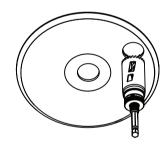
*NOTE:* Avoid the three flanges on the locking nut when drilling an offset hole though the mounting plate's surface. Rotate the nut or relocate the drilling location to avoid these three flanges.
