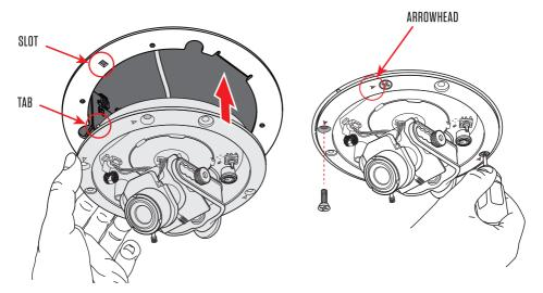
Make any required adjustments to the camera, then install the dome top as detailed in the install guide for the camera.
