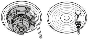
Note: When drilling an offset hole through the mounting plate, be sure to avoid the three flanges on the locking nut. If necessary, rotate the nut or adjust the drilling location to prevent interference with these flanges.
